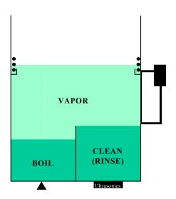
is utilized, it is necessary to adjust temperature control settings. Alcohol may be extracted from the system if large quantities of water are introduced to the vapor degreaser. Desiccant drying is recommended in the condensate return loop to prevent alcohol loss.
